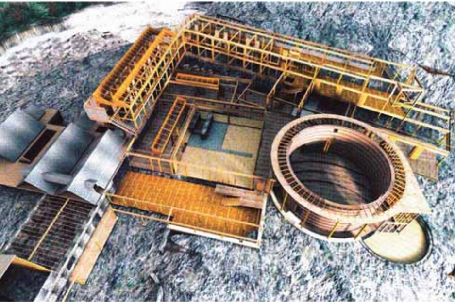
Below: the timber frame will extend throughout the WISE buildings
